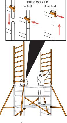
Fit two pairs of diagonal braces in opposing directions between the 6<sup>th</sup> and 10<sup>th</sup> rungs and the 10<sup>th</sup> and 14<sup>th</sup> rungs. Locate a trapdoor deck on the 12<sup>th</sup> rung.
