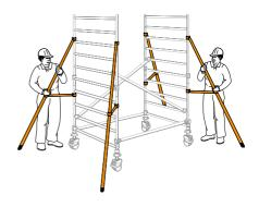
Fit a temporary deck on the lowest rungs. Fit a trapdoor deck on the 8<sup>th</sup> rung (2.0m) on one side of the tower. Ensure that the trapdoor is positioned with the hinges towards the outside of the tower as shown. Climb the end frame below the trapdoor on the inside of the tower, and from within the protected trapdoor position, fit horizontal braces on the 10<sup>th</sup> and 12<sup>th</sup> rungs (in that order) on both sides of the deck.
