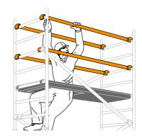
Continue the procedure until the required working height is reached, adding additional pairs of end frames, diagonal braces and fitting trapdoor platforms, as shown on previous steps. At every platform level, add horizontal braces as guardrails at 2 and 4 rungs above the platform (in that order) on both sides of the platform (as shown in **Step 5**).
