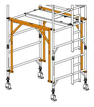
If end walk-through access is required at the base of 2.2m, 4.2m, 6.2m, 8.2m, 10.2m or 12.2m platform height, 1450 wide towers, walk-through frames may be used.
