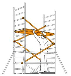
Climb up the inside of the tower and from the protected position of the trapdoor, fit horizontal braces as guardrails (on both sides) to the 14<sup>th</sup> and 16<sup>th</sup> rungs (2 and 4 rungs above the platform in that order).
